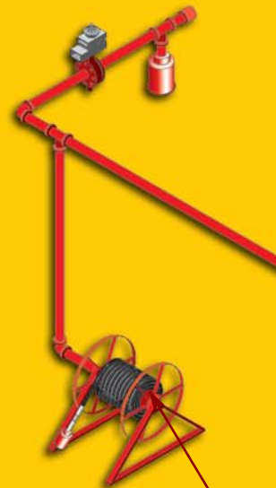
Hose Reel Station Available with 50, 100 or 150 (15, 30 or 46 m) of Hose
